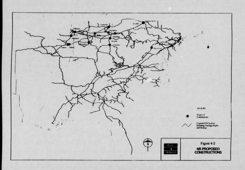
NS proposes constructing 14 new connections (Figure 4-2), six of which would be built on existing railroad right-of-way and eight of which would require the acquisition of additional right-of-way. The proposed rail line construction projects would be in Illinois, Indiana. Maryland. Michigan. New York and Ohio.
