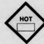
**Loaded** "Elevated Temperature Material" cars must be handled only with proper hazardous material documentation (See HazMat Timetable Rule E). For example:
