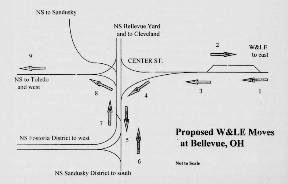
(1). At Yeomans, W&LE would use the siding to run the engines around the train (2). During this time, no other trains could enter or exit Bellevue using the W&LE line.
